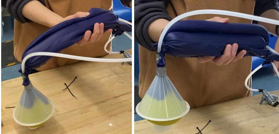
Figure.6: Actual shape of the fabric pneumatic artificial muscle with a gripper.
